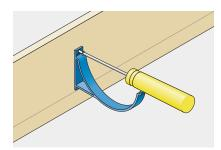
Generally position fascia brackets at 900mm centres in accordance with BS EN 12056-3:2000. Fix brackets with two No 12 x 38mm round-head screws.
