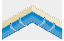
Offer angle pieces and outlets to the fascia. Lower gutter sections onto the brackets leaving a 4mm expansion gap between gutter sections and allow sufficient clearance for the gutter joint.
