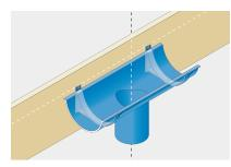
Plumb line outlet positions with gullies at ground level.
