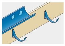
6. Clip gutter sections into brackets.
