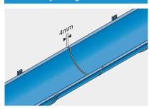
7. When joining gutter lengths, allow for a 4mm expansion gap.
