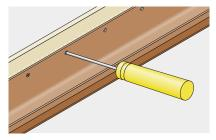
Fix all components and gutter lengths direct to the fascia with a single roundhead screw through the back edge at 900mm centres. Drill 8mm holes 18mm from the top edge.
