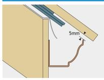
Using a straight edge or ruler, shim gutter brackets with 5mm clearance so that the last roof tile or slate will align with the mid point of the gutter.
