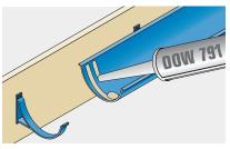
Apply two 6mm beads of Dow Corning 791 low-modulus Type A silicone sealant to the ends of gutter profiles and fixing hole. Silicone sealant must be applied only to completely dry surfaces.
