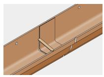
Tool-off displaced silicone sealant to the inside of the gutter joint. Tighten fixing bolts. Cone-off bolts and any other potential leakage points with sealant. Allow to cure for 24 hours.
