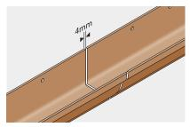
6. When joining gutter lengths, allow for a 4mm expansion gap.
